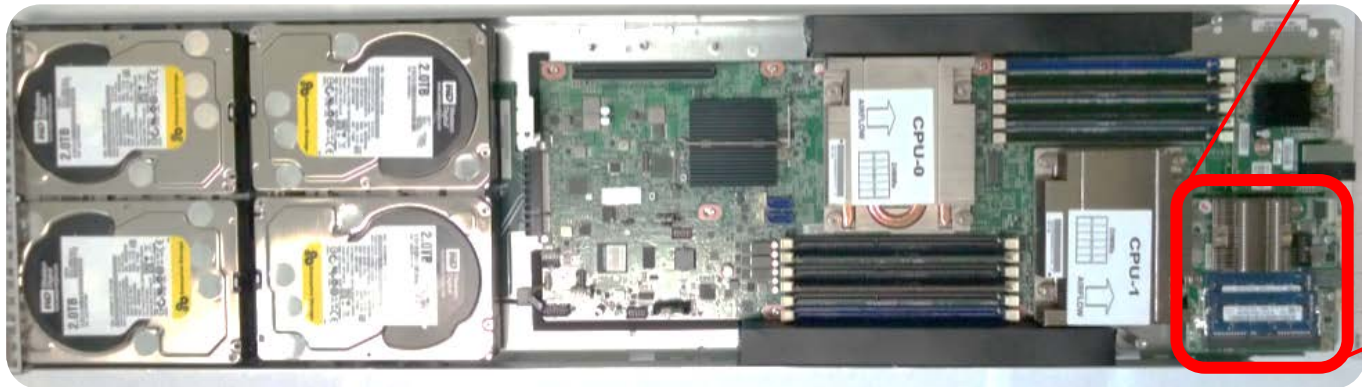
Data Center Server (1U, ½ width)
